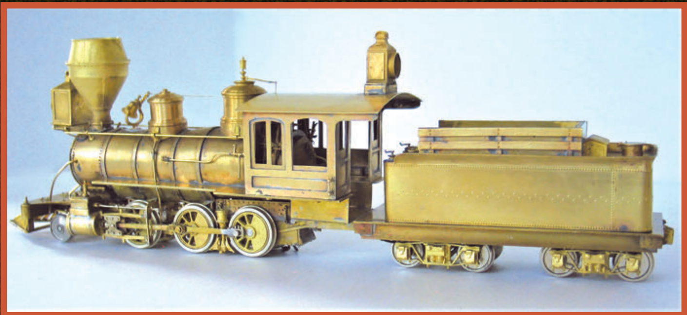
Below: Left side still needs to have the pipe from the injector to the tender installed.
