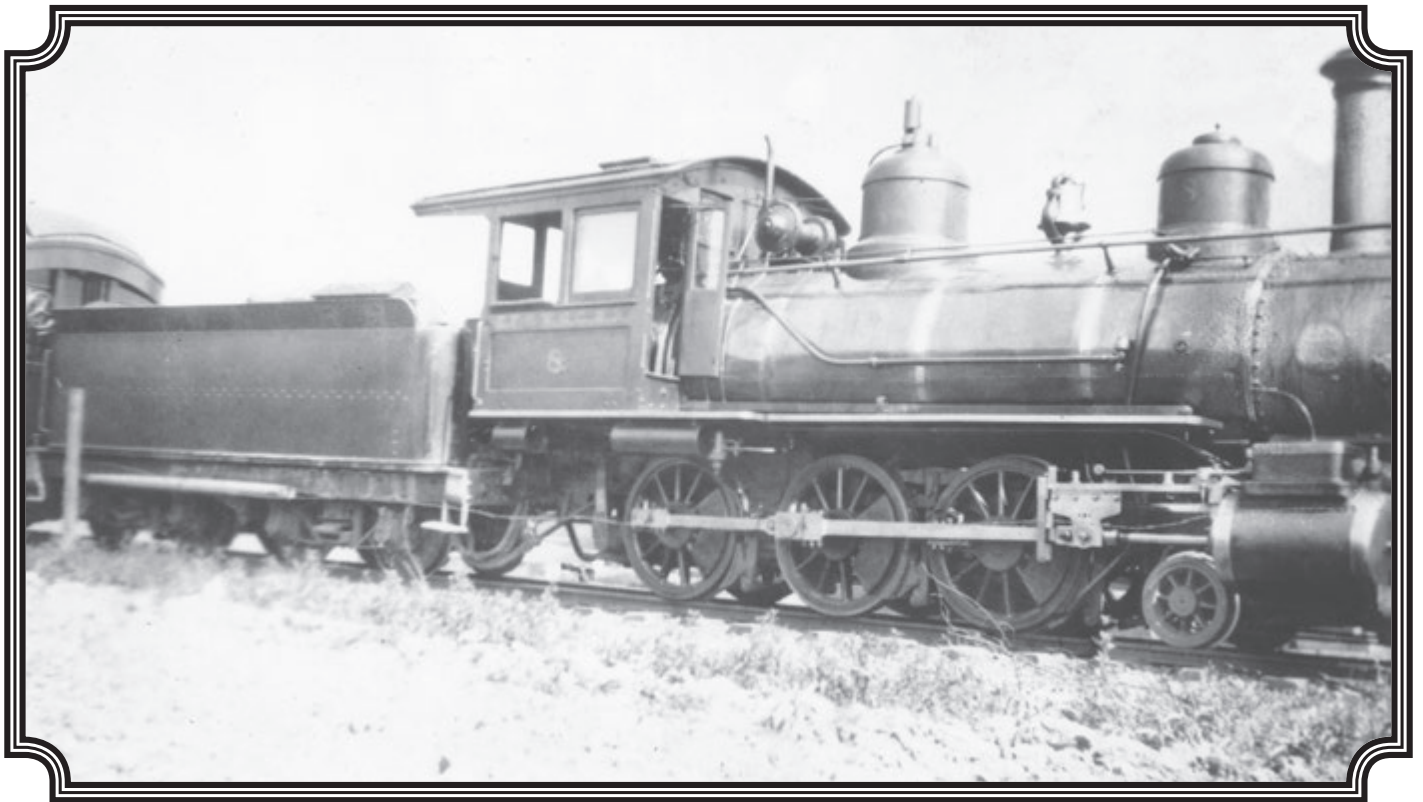
Above: Number 8 is shown here after the bell and sand dome were switched around in 1915. The drivers appear to be fairly light weight, indicating that the locomotive was well balanced and built for speed, not pulling power. The jacket bands and cylinder heads were polished brass. Photo, collection Mike Dowdy.
