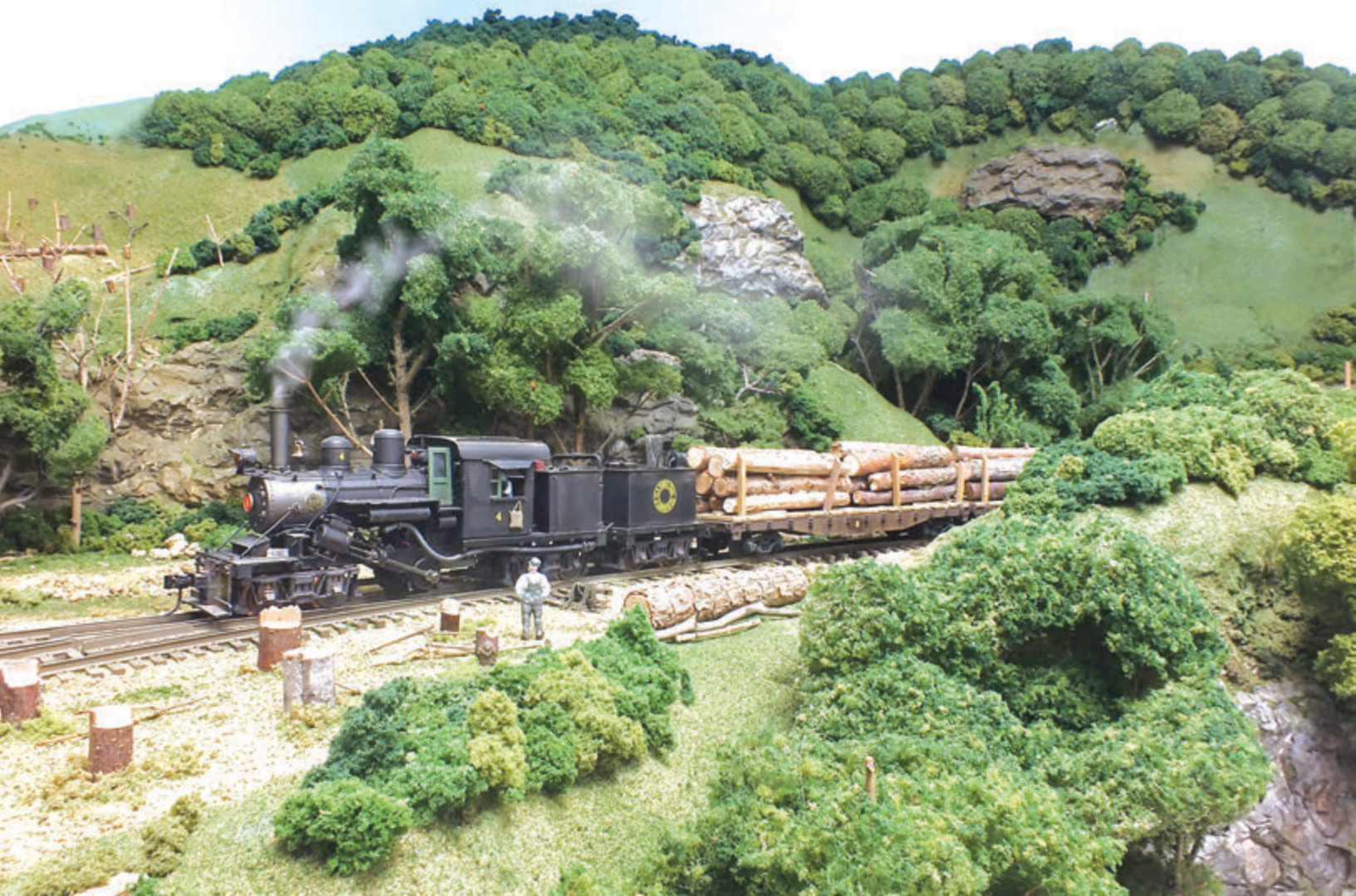
Above: While there are no photos showing the complete locomotive, records show that at one point a 3-truck Climax #4 was rostered on the ERC&L. The author built this model of the engine by modifying a Bachmann On30 locomotive. It is shown here with a string of loaded log flats ready to depart for the sawmill at Swandale.
