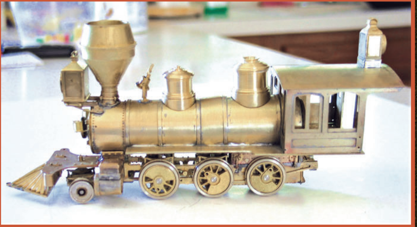
Above: This early construction photo shows drivers, boiler and cab temporarily positioned on the frame to measure for frame extensions and lower cab sides.
