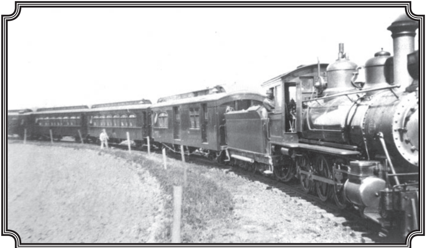
Below: The ET&WNC purchased an all vestibule passenger car set from AC&F in November 1917. The full set plus #8 and the AZALEA parlor car sit on the coach shed track around 1918. These heavy cars proved to be too much for the small Ten Wheeler. Photo, Mike Hardin Collection.
