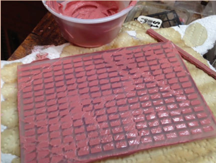
Above: This mold, designed for military modelers, was used to cast individual brick for the engine house floor. The bricks were cast in colored casting plaster.
