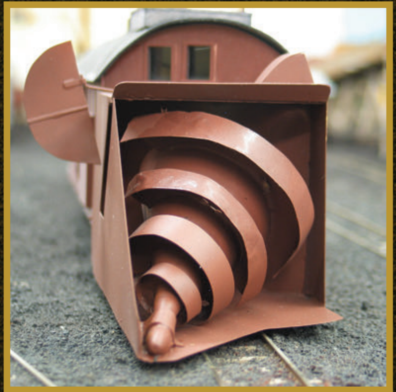
Right: Front view showing the auger and the snow deflector on the upper left of the housing.
