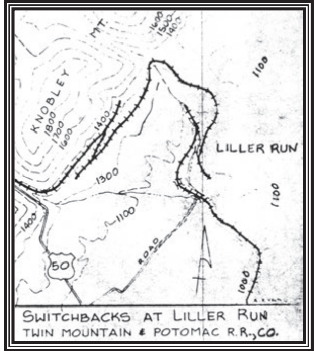
Below: The roughest part of the route of the TM&P was the descent from the pass on Knobley Mountain down to Burlington. The elevation lines tell the story of the grades the railroad had to deal with every day. Photo, collection of Larry Smith.
