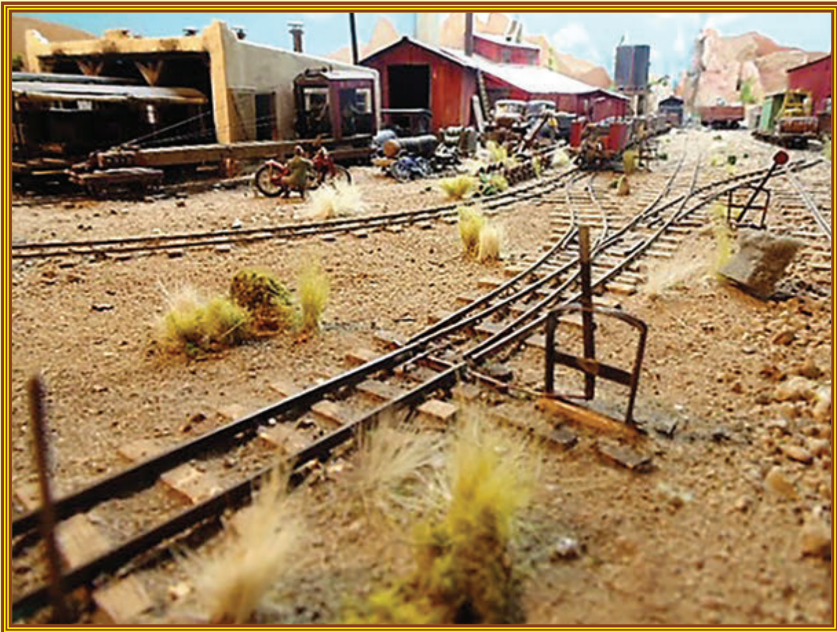
Left: The Terlingua, Glenn Springs & Boquillas still uses stub turnouts with harp switch stands.
