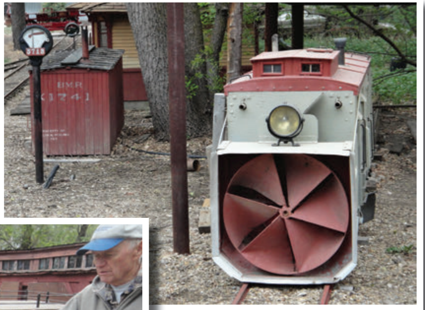
Right: This rotary snow plow works and is used to clear snow off the tracks in winter.
