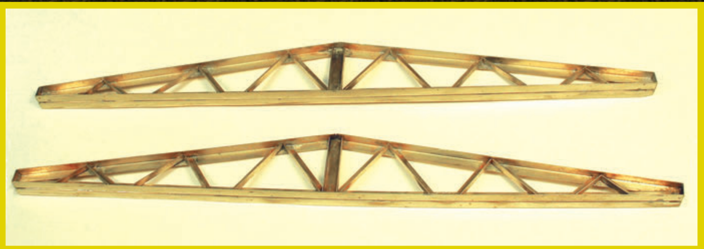
Below: Finished side frames. Note the end caps and the additional angles soldered to the backs of the top girders.
