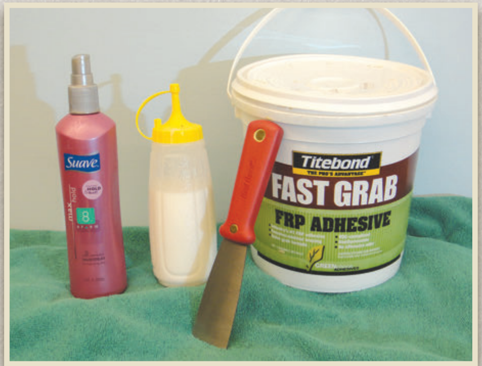
Above: This is the construction adhesive, water sprayer, and diluted glue dispenser used in completing this project.
