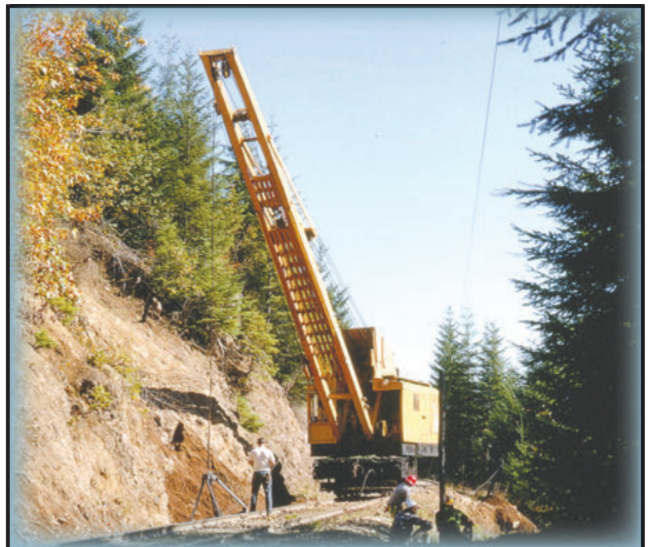
Below: A Simpson Timber Company Clyde doing some ditching on the line to Camp Govey.
