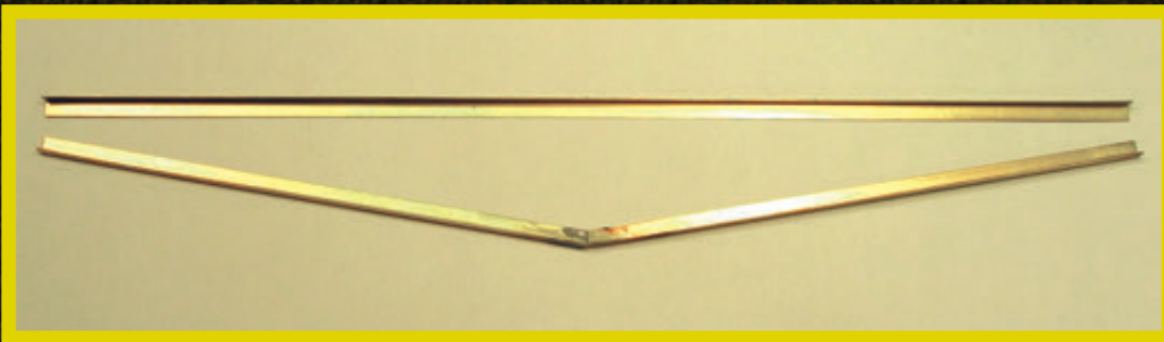
Left: Top and bottom angles ready to be soldered together to start the side frames.
