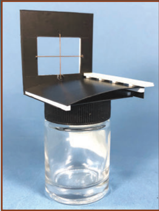
Above: This is the front view of a permanent mask. It is meant to simulate the roof of a caboose with part of the roof walk showing. The brass wires in the window are meant to simulate the mullions in the cupola window. All the details here are what the camera would see in the foreground as it looks through the window.
