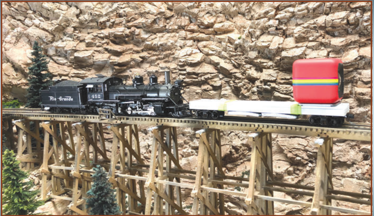
Above: Before committing to the new camera car design, I took it for a test ride on my layout. It was setup like the Micro Trains flatcar. In this photo, I was experimenting with weight and stability. The top of the car isn't yet glued in place, and I've hung weights under the car. I thought the lower center of gravity might help stabilize the car but, in the end, it didn't make any difference, so I only used the weights buried inside the car.
