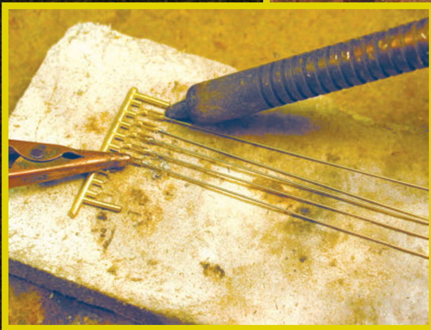
Left: The soldering machine probe and ground clip are used to solder brass wire into one end of the turnbuckle. A soldering iron could also be used.
