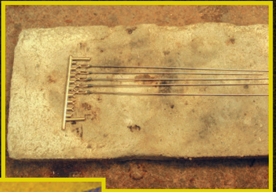
Right: As described in the text, solder paste has been applied to the turnbuckle castings with a straight pin.
