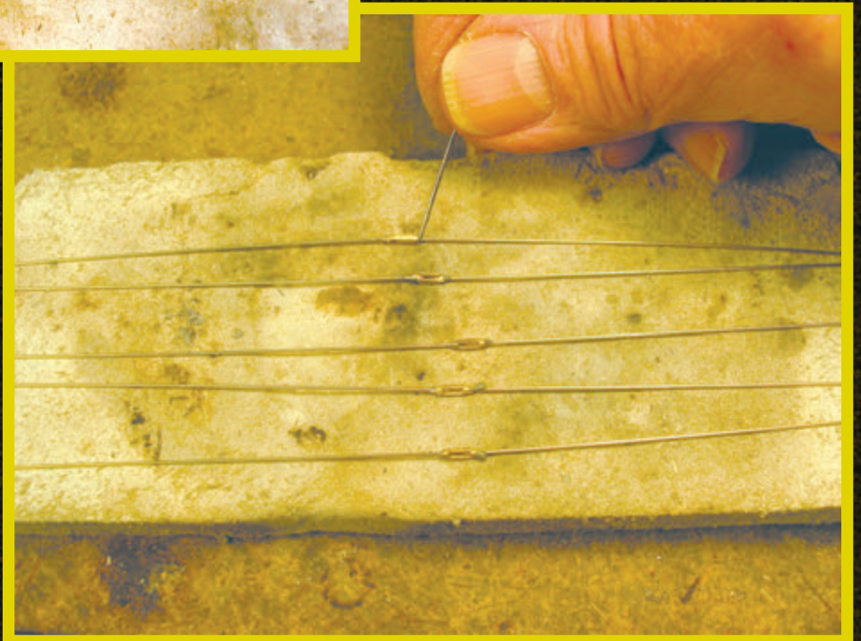
Right: Previously soldered turnbuckle castings have been removed from the sprue and solder paste is applied to the remaining end. The paste is placed at the end of the casting and the heat will cause the solder to flow around the wire, resulting in an open turnbuckle. 🛠️
