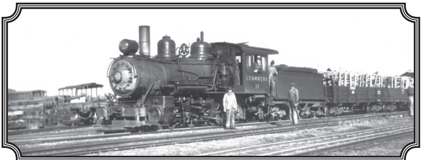
Below: During the early years of the Great Depression, the new rayon plants at Elizabethton kept the narrow gauge busy, and profitable. The fire hazard was high there, so the locomotives had their trademark cap stacks removed and replaced with a straight one that had a flip up spark arrestor attached. The cowcatchers were removed as well, to aid switching so many standard gauge freight cars. Wayne Arnold Collection.
