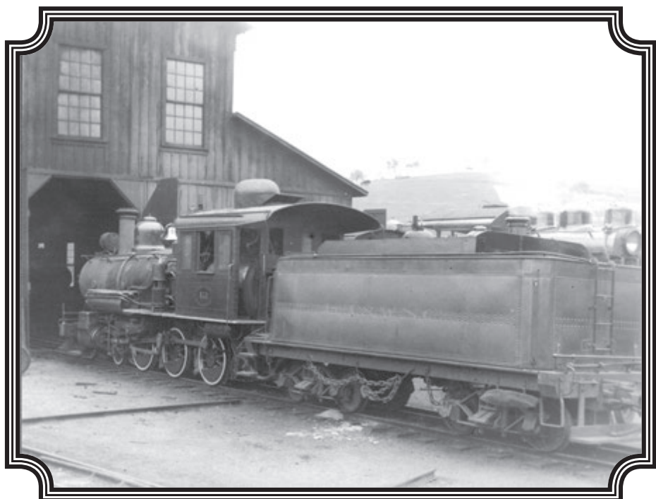
Below: Number 12 is showing her "tender behind" in this view at the Johnson City engine house around 1940. The gold leaf lettering was prone to fading so after a couple of years, it was all but illegible. Note the backup light in the right corner of the tender, where it would most benefit the engineer. Ken Marsh Collection.
