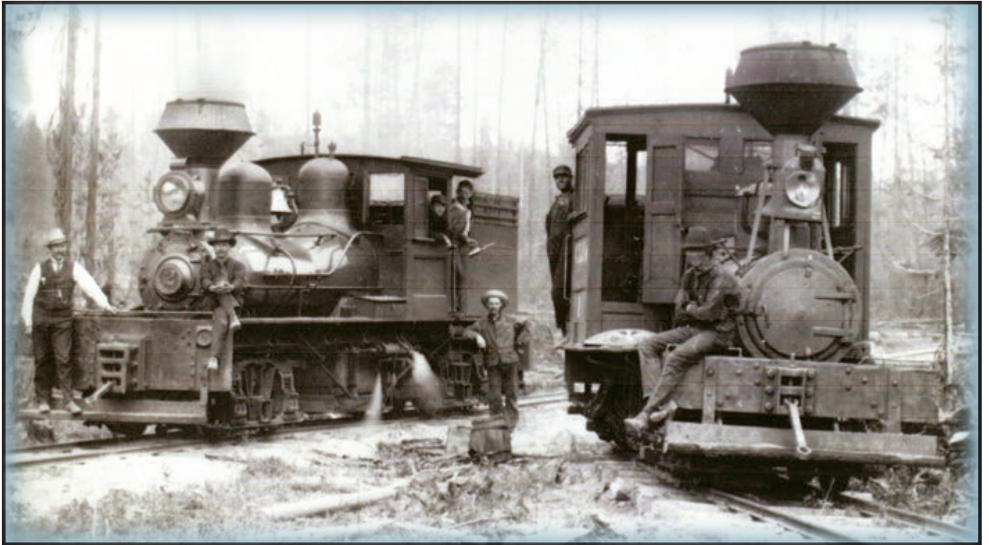
Above: Here are Shays #2 and #1. Number 1 was the oldest Shay in the West having been built in 1883 for Henry Sherry and Company of Vesper, Wisconsin, in 1883. It was an A-11 class Shay. Photo, Robert Pearson collection.
