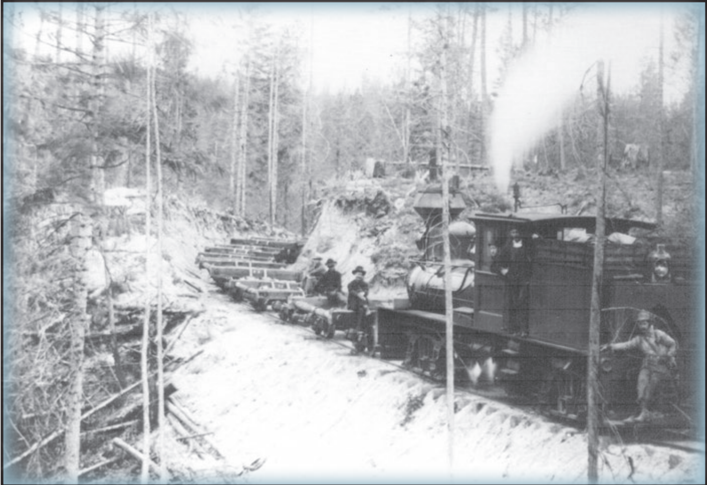
Below: A train heading out into the woods with a string of empties. The company used Russel Wheel and Foundry Co. #2 pattern cars. Photo, Robert Pearson collection.
