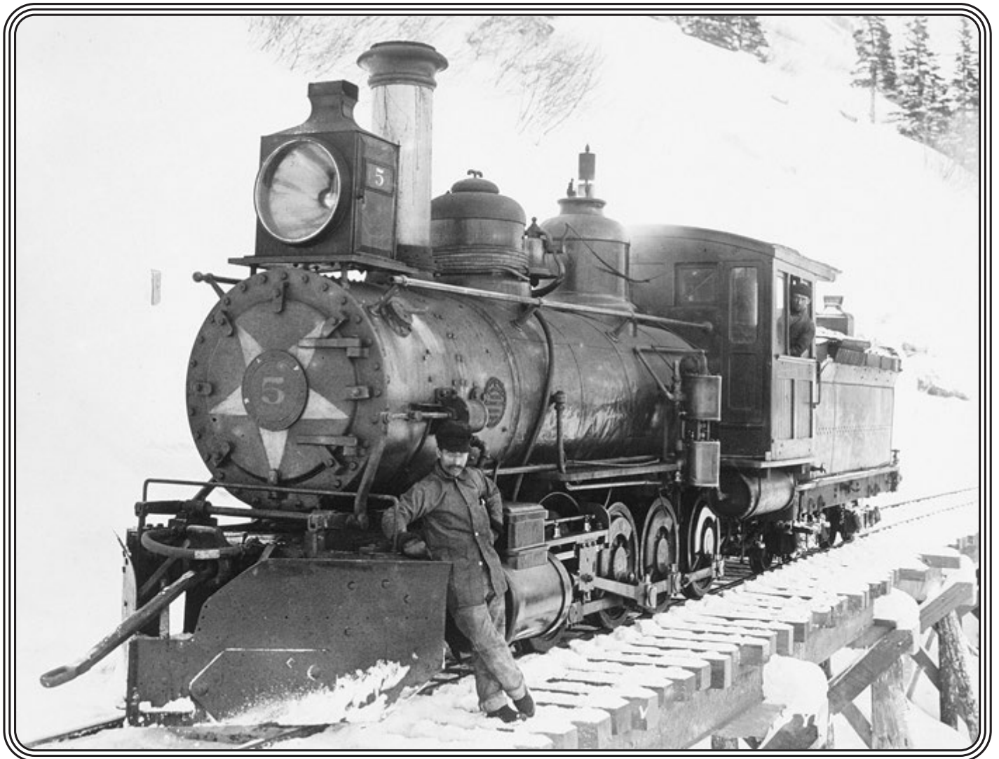
Above: White Pass & Yukon Route #5 has stopped on a trestle for a portrait sometime before the 1900 renumbering, when it became #55. The shop or crew has painted an upside-down star on the smokebox front. Note the snow plow with flangers, and the flanger actuator mounted to the side of the smokebox. Photo by E.A. Hegg, Bruce Pryor collection.
