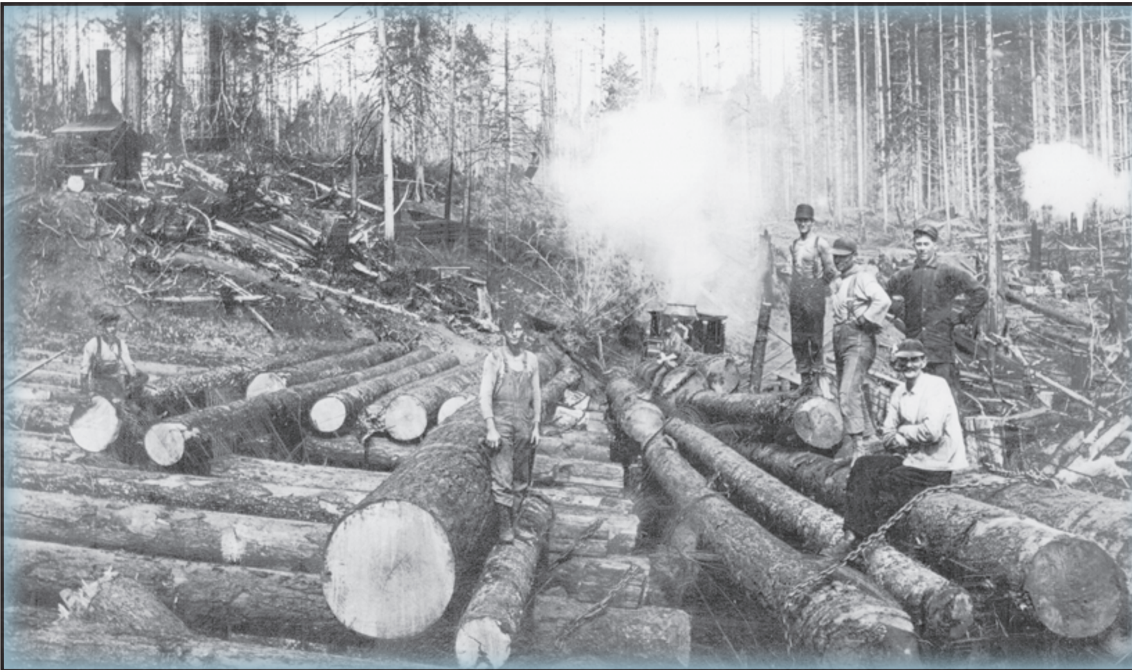
Above: Loading logs on disconnected cars at roll way landing with two steam donkeys visible. Photo by M. Lee, John Labbe collection.
