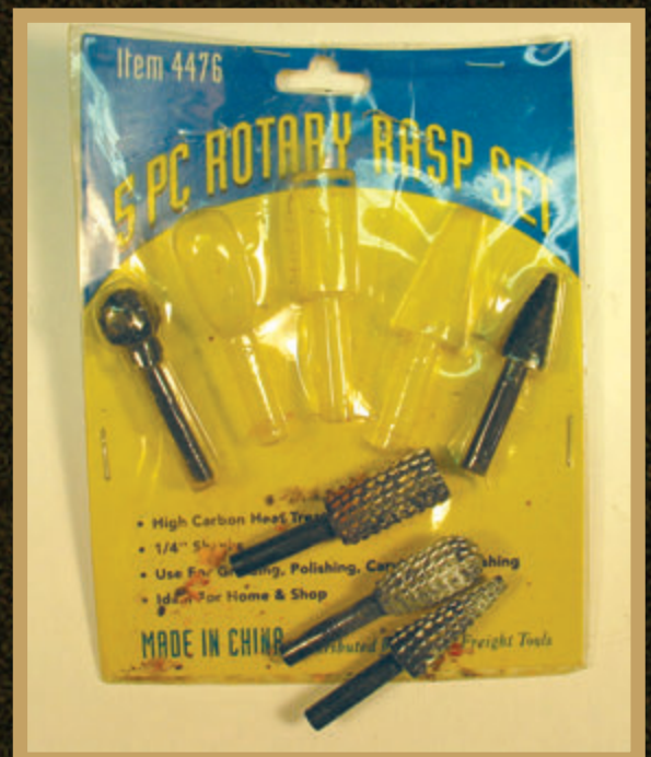
Right: This rotary rasp set was used in an electric drill to grind down the protruding stones in the wall castings.
