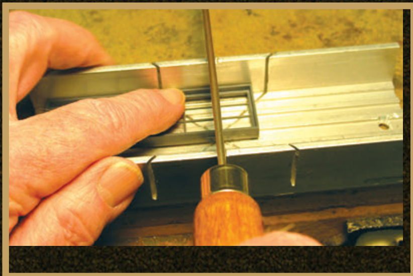
Below: I put a new, sharp blade in my Zona saw to minimize breakage when sawing pieces out of the window castings. It worked.
