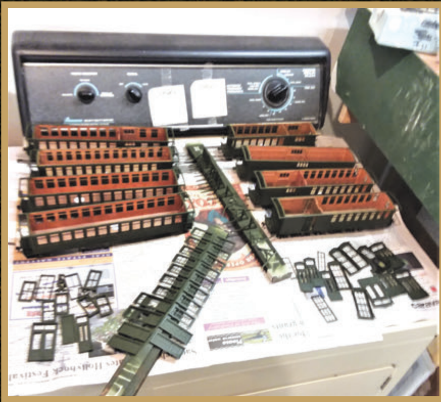
Above: This unusual photo is an example of my model assembly line production approach. Whenever possible, I try to combine working on similar items rather than do them individually, whether construction or painting. I had a few passenger cars ready for painting at the same time I needed to paint the details for the depot. Because Floquil Coach Green is no longer available, I use Model Master Dark Green on my passenger cars. I keep a lot of bottles on hand, so it seemed natural to paint the depot trim the same color. I mounted the pieces on strips of masking tape fastened to 1- x 2-inch wood strips for ease of handling as shown in the photo. After a busy few hours of airbrushing, the top of the clothes dryer was used to allow the paint to set for a few days.
