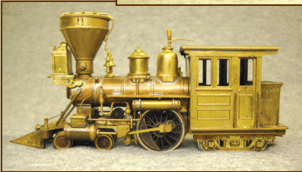
Left: Left-hand view of the completed locomotive. Boiler was turned from solid brass with a slot milled out of it to clear the drive worm. The cab, fuel bunker, domes, bell, headlight, whistle, and stack are some of the many commercial parts that were used to keep the project from getting out of hand.
