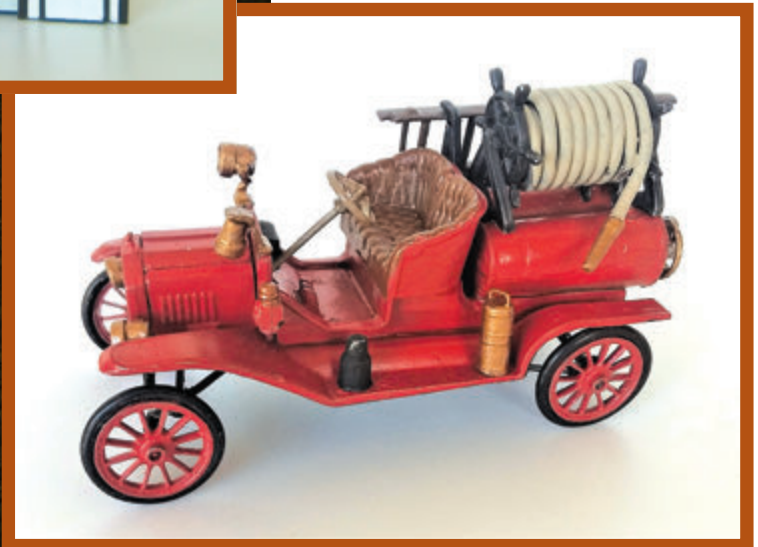
Right: This interesting fire truck is from National Motor Co. The company produced a series of white metal kits based on a Model-T chassis that are now available from Wiseman Model Services. The hose is solder wrapped around the reel and painted with craft paint.
