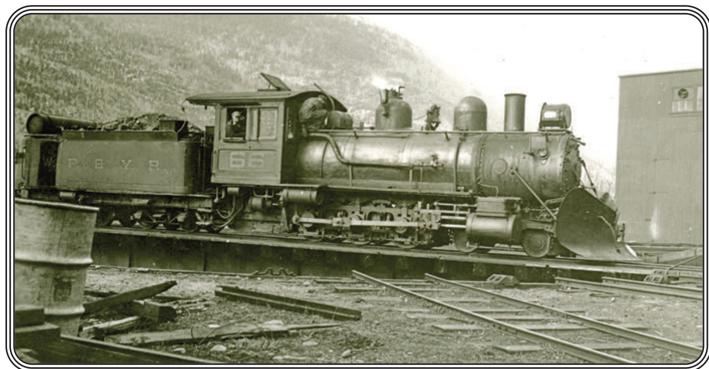
Below: WP&YR #66 is on the Skagway turntable wearing her snowplow, while a crewman makes an adjustment to the dynamo. Note the smooth domes used on #66 and #67. The very tip of the plow appears to have a small amount of snow stuck to it, but the locomotive doesn't have the winter coal boards or cab curtains installed. The 59-class steam dynamos all seem to have had sheet metal covers; probably a winterization innovation developed by the WP&YR shops. A close look at the pony truck shows the flanger and some of the related linkage. Photo courtesy Skagway Museum, #01.360, high resolution scan by Chuck Morse.
