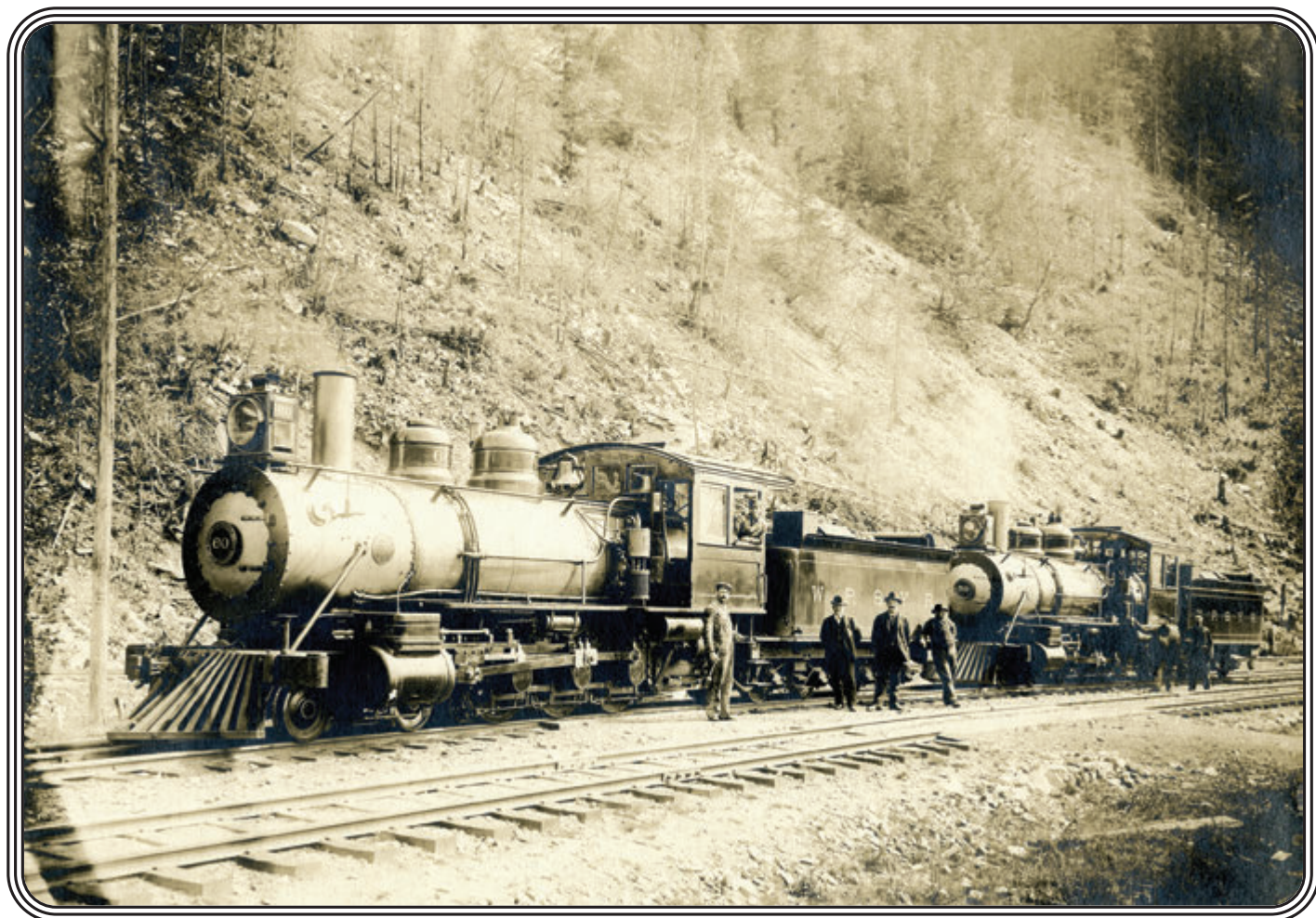
Above: WP&YR locomotives #60 (left) and #59 (right) appear brand spankin' new here, and very possibly are. They don't have the snowplow brackets on the smokeboxes yet or the second air pumps. Photo by H.C. Barley, courtesy the Skagway Museum, Talbot-040, high resolution scan by Chuck Morse.
