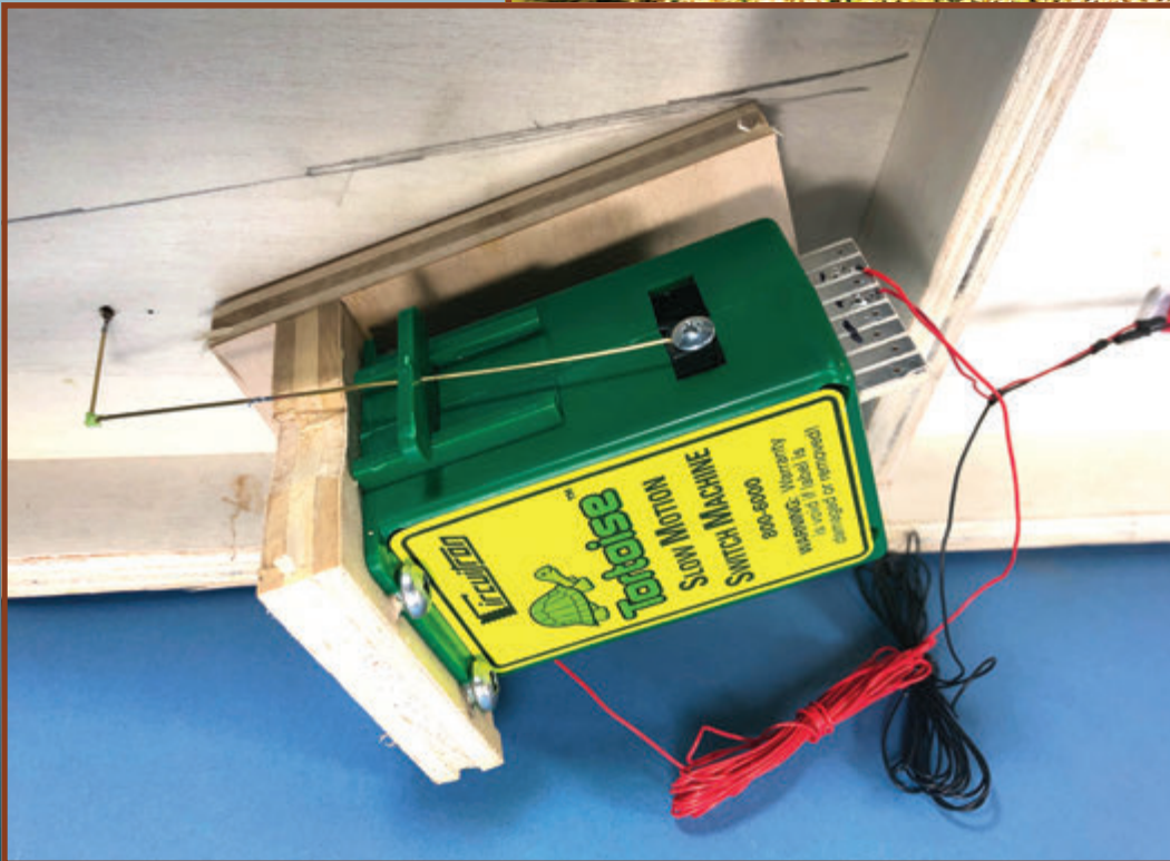
Left: I mounted a Tortoise switch motor on its side to control the rod that will be used as a car stop on the coal pocket trestle. A switch that's built into the Tortoise is used to turn the power to the DCC decoder on and off. When the rod is in the up position, the decoder gets power from my DCC system. When it's down, the power is off. This in turn toggles the fusee LEDs on and off.
