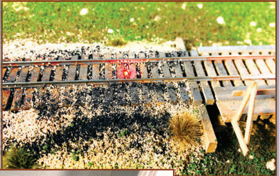
Right: The LEDs were placed between the ties on the approach to the coal pocket trestle. These will warn my operators that the car stop is in the up position and to be careful spotting cars at the coal pocket. Combining the two separate firebox flicker effects creates a pleasing effect that simulates a fusee burning. I tried to set the LEDs below the rail height so that they wouldn't get damaged when I'm cleaning the track.
