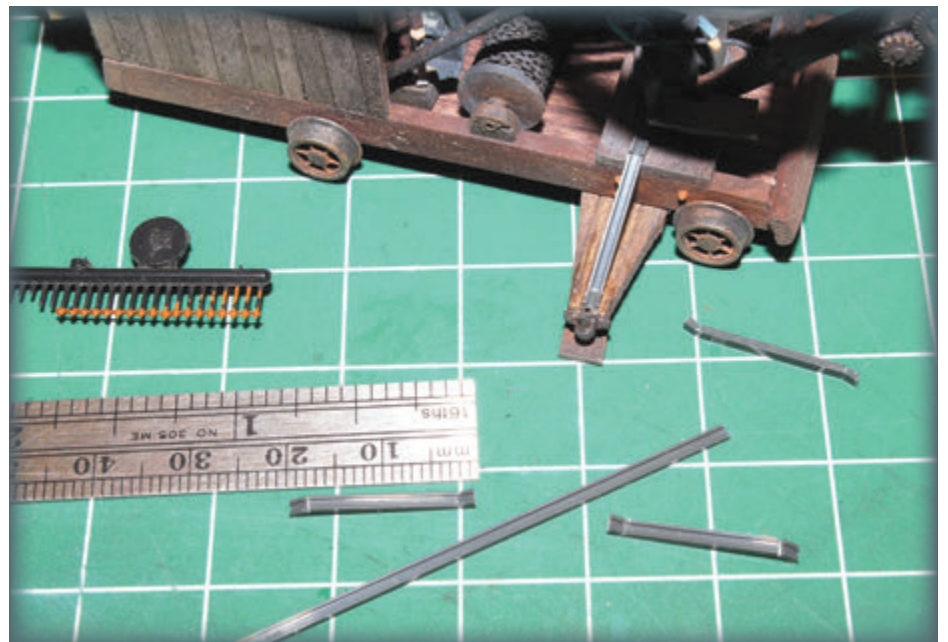
Below: On the prototypes, lateral ground support braces were made from wood and ran the full width of the chassis. They were reinforced by steel (plastic on the models) channel. The pads on the supports could be moved to level the machine.
